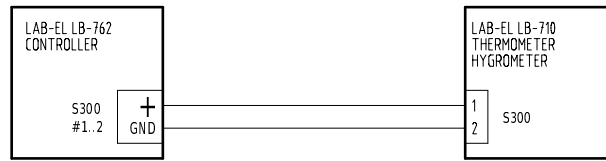
Rysunek 3.5: Scheme of connection of LAB-EL LB-710 type meter
