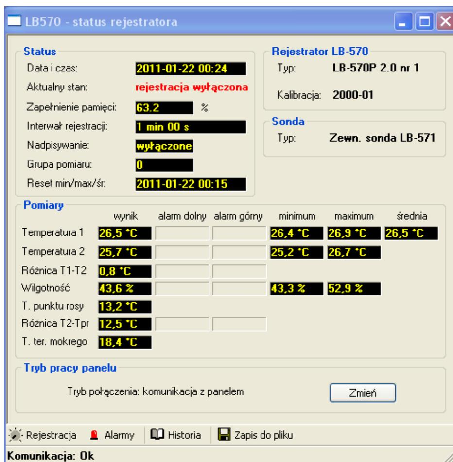
**Fig. 4 Exemplary view of the (status)window in the LOGGER program, after connection to the hytherograph LB-570P**
