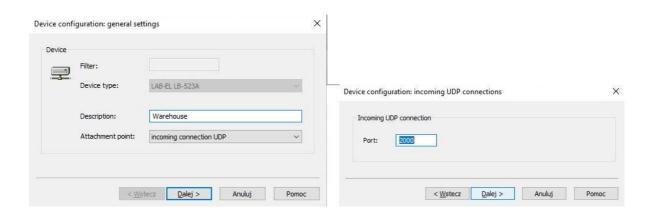
The 'Descriptive name' field is any name under which all LB-523A will be grouped, transmitting data to the port number entered in the 'Port' window. LBX configuration is made only once for all LB-523A, which are to be grouped under one name (e.g. for 10 LB-523A, configuration is done only once).
