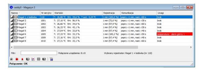
The picture above shows the main window of the program with eight LB-523A recorders (7 thermohygrometers and 1 thermohygrometer with an external thermometer for measuring the temperature of any medium).
