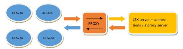
The scenario is as follows: LB-523A sends a request to the proxy server (upper orange arrow), the proxy server forwards the request to LBX (upper yellow arrow), the LBX server responds to the request received from the proxy (lower orange arrow), the proxy server forwards the response to LB-523A (lower blue arrow).
