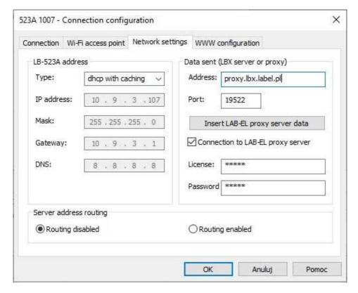
For a connection that uses an intermediate proxy server, the required parameters are:
