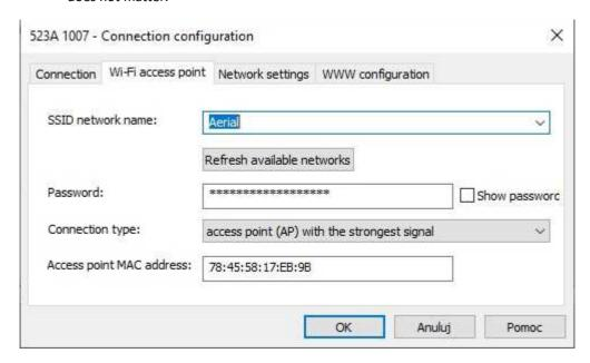
The 'Refresh available networks' button will scan available WiFi networks and display a list of found access points (APs). Pointing to the selected AP from the list will rewrite its name (WiFi SSID network name) and MAC address to the appropriate fields in this window.
