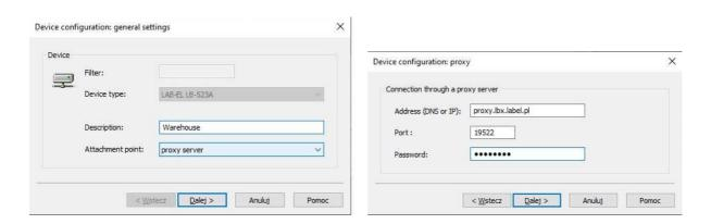
The 'Descriptive name' field is any name under which all LB-523A will be grouped to the proxy server. The LBX configuration is made only once for all LB-523A, which are to be grouped under one name (e.g. for 10 LB-523A, the configuration is performed only once).
